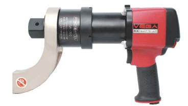
A Pneumatic Torque Wrench is an air motor driven planetary gear box having a very high reduction ratio. The gear box is provisioned with a reaction arm to absorb the torque reaction. Unlike impact wrench a pneumatic torque wrench is driven by continuous gearing and hence has no noisy and hazardous hammering. This is why a pneumatic torque wrench has an excellent accuracy and repeatability. Pneumatic torque wrench offers following significant advantages:
